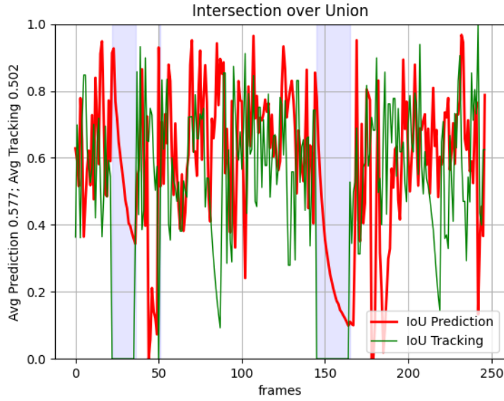
Figure 4.41: IoU for the occlusion during flight case: The UAV is occluded twice during the experiment, indicated by the blue-shaded areas.
