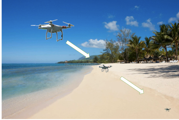
Figure 4.1: The drone begins at its starting position A in the top left corner and ends at B at the bottom right. Due to its movement away from the observer, it is scaled accordingly.
