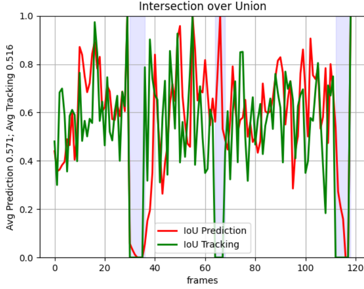
Figure 4.19: IoU between Ground Truth and Prediction / Tracker for the Inaccurate Tracker case: Due to the noise the prediction sometimes follows the wrong direction, as indicated in the first jumping period. This results in a poor performance. However, depending on the current flight path, the prediction may sometimes even drastically improve, as seen in the second period. The third is the expected case, where the IoU falls during subsequent time steps.
