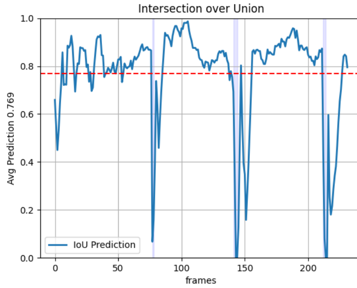
Figure 4.36: IoU between ground truth and Prediction for inaccurate tracker case: The faulty tracker jumps to other parts of the screen during time periods shaded in blue.
