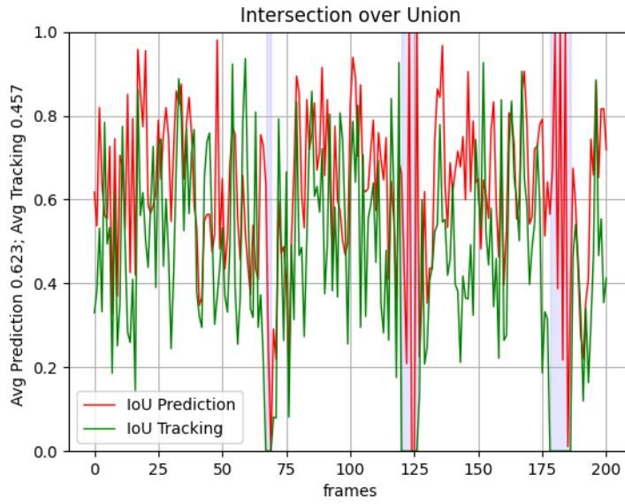
Figure 4.37: IoU between ground truth and tracker/prediction for inaccurate tracker case: During the period, where the tracker has jumped, the prediction is still able to follow the ground truth position for a few frames.
